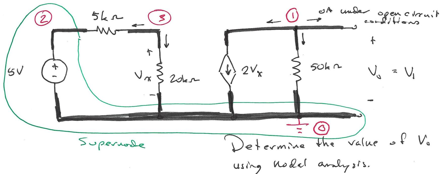
$V_2 = 5V$  (constraint eqn. for the supernode)
