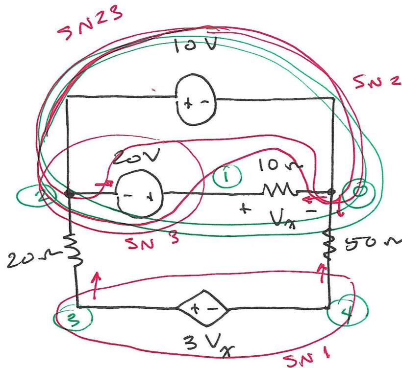
For  $SN1$ :  $\frac{V_3 - V_2}{20} + \frac{V_4}{50} = 0$  (KCL)
